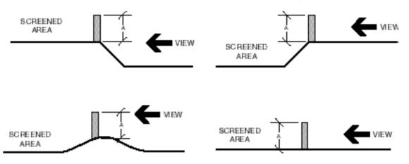
NOTE: A Screen Height Measured from Finished Grade.
